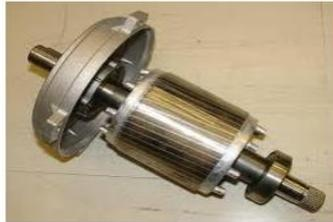
Figure 7.3 Squirrel cage rotor.
